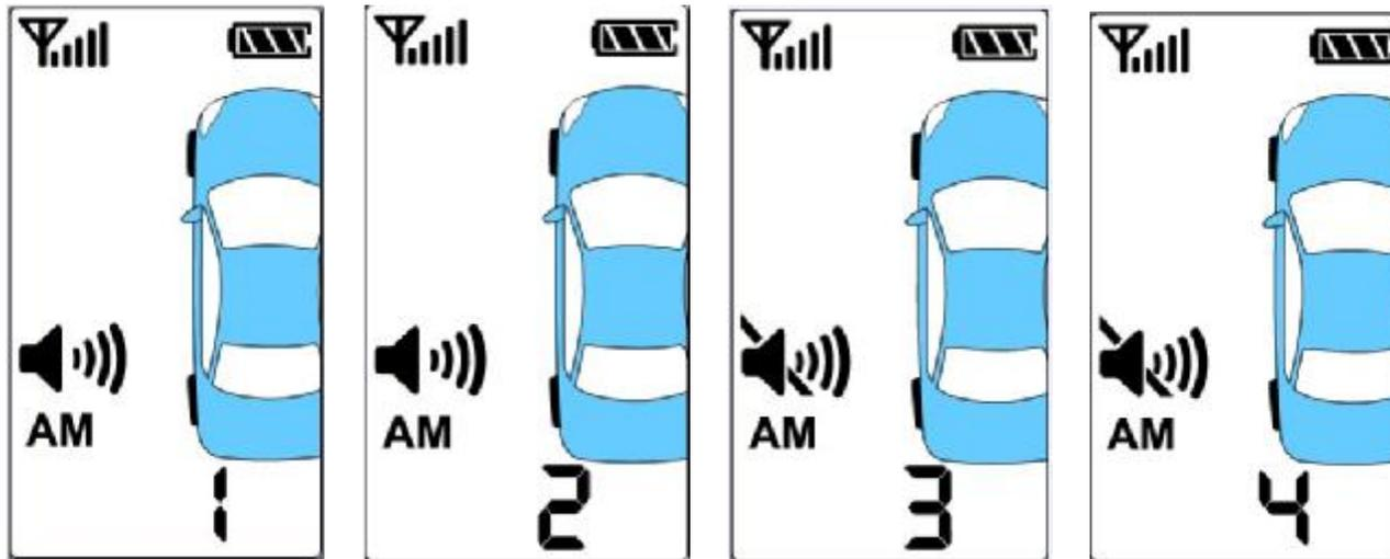
Mode 1: The remote beeps once and vibrates: this indicates “Beep ON & Vibrate ON”.
